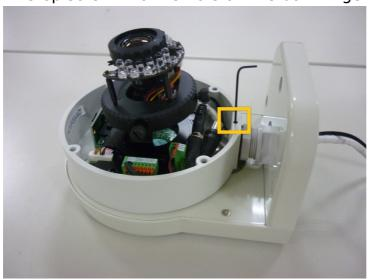
8. Close the dome cover, and use the 3 screws to fix the L-shaped bracket on the wall.
