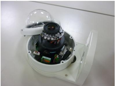
2. When putting the camera on the L-shaped bracket, please refer to the four screw holes marked in orange.
