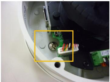
5. Make you external cables (power cable, ethernet cable.etc) through the waterproof connector and the hole of the bracket, and then connected with the camera.
