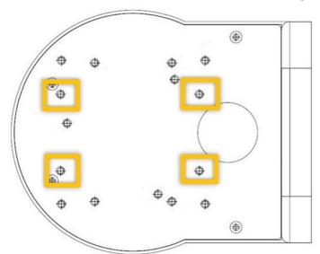
3. Apply the black o-rings on the screws. Without the o-ring, water may seep into the camera through the screw holes.
